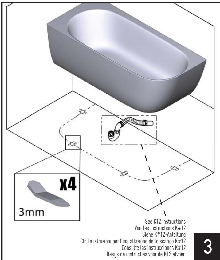
Install bathtub K12 waste drain into floor surface. Position the bathtub spacers (x4) as shown and ensure bathtub drain hole is aligned with waste drain before positioning bathtub.
