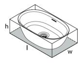
$l = 544mm & weight = 6kg \\ w = 325mm & capacity = 9L \\ h = 153mm &$
